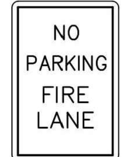
NO PARKING FIRE LANE 12" x 18" RED ON WHITE REFLECTORIZED 7'-0" MOUNTING HEIGHT (LR7-22) SIGN-FL NOT TO SCALE
